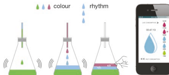
Figure 3. In the Water Amplifier the amount of drops signals the current use of electricity
