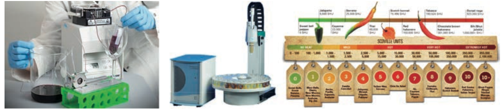
Figure 7 - The proposed tools for analysing taste qualities: the electronic Tongue and the Scoville Scale ®
