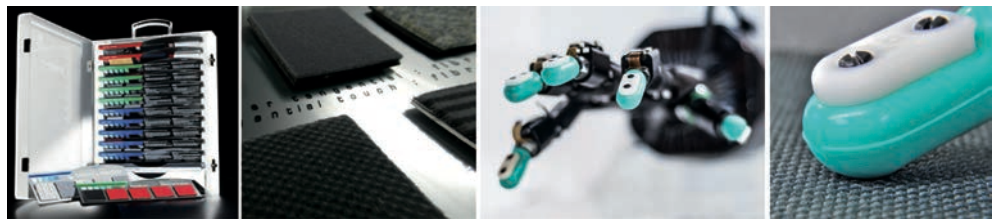
Figure 6 – The proposed tools for analysing touch qualities: SensoTact ® and BioTac ®
